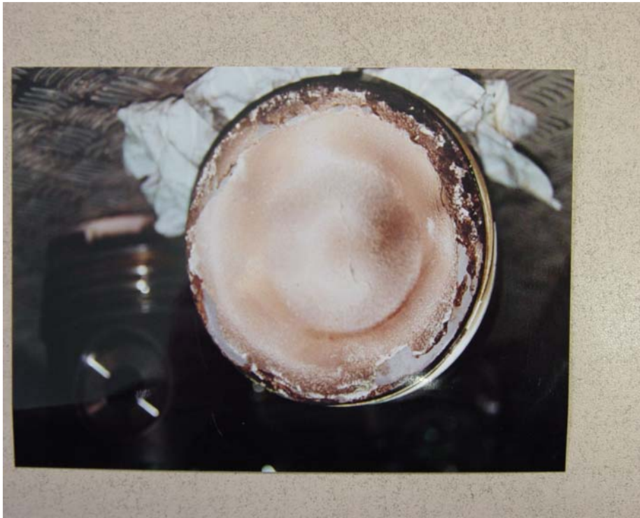
Photograph 2: SiO 2 and silicate Deposits on piston crown and rings
